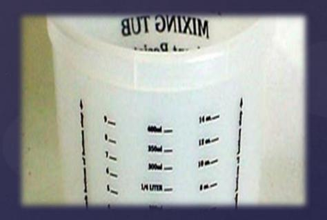
Stone Bond Epoxy is a three to one ratio. <u>Important:</u> DO NOT VARY FROM THIS MIX RATIO.
