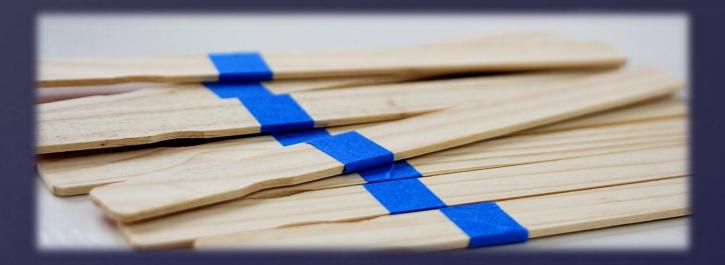
Mix for two minutes with a flat stirrer, scraping the sides to ensure proper mix. Let stand while loading mixer.
